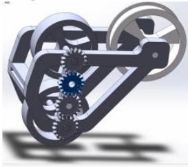
Fig.2 Head, tongue ejection and grasping mechanism
