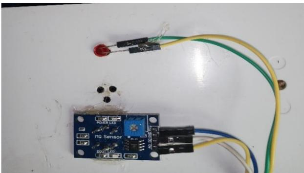
Fig. 8 Addition of MQ-5 gas sensor and LED indicator to the entire circuit
