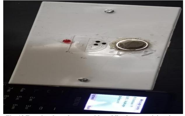
Fig. 13 Functional gas detector with mobile phone receiving short messages service signal via GSM module
