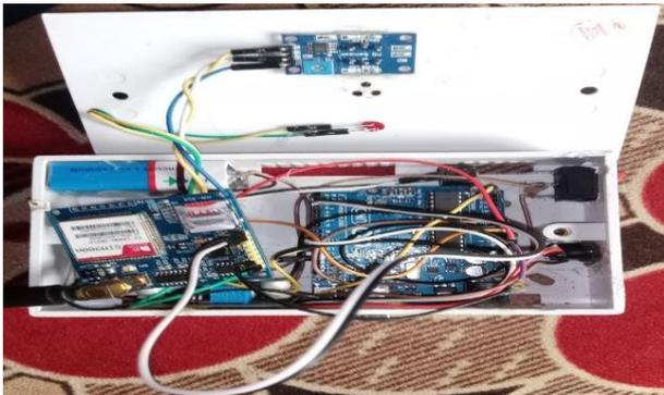
Fig. 7 Integrating GSM module with other devices to implement SMS notification
