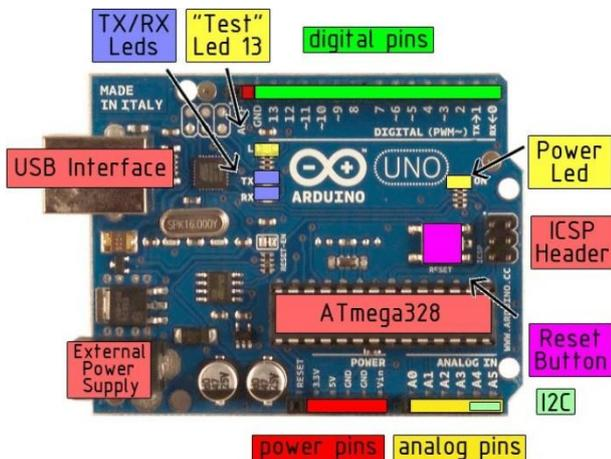
Fig. 2 The block diagram of the microcontroller
