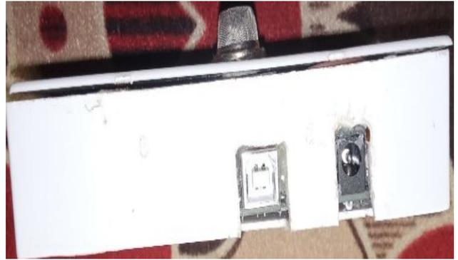
Fig. 10 Creating access point for microcontroller port for easy access to load program via universal serial port
