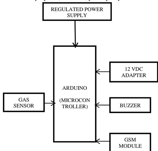
Fig. 4 Microcontroller System Architecture for smoke detection
