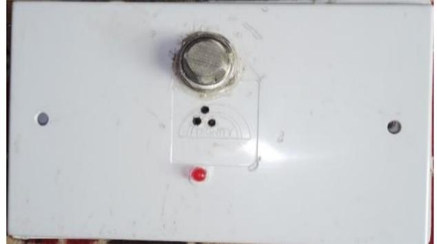
Fig. 12 Complete gas leakage detector device ready and encased in a parterres
