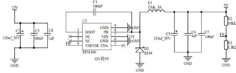
**Fig. 12 TPS5430 Buck circuit**
