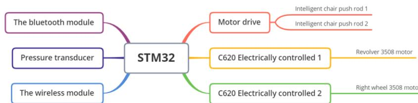
**Fig. 5 Electronic control component**
