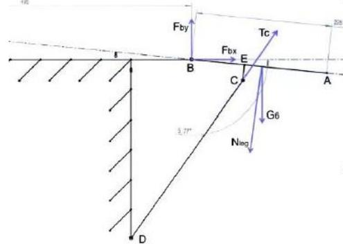
Fig. 11 Leg brace - mechanical model
