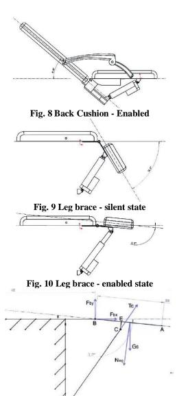
Fig. 11 Leg brace - mechanical model
