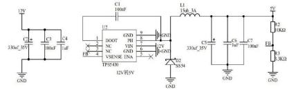
Fig. 12 TPS5430 Buck circuit
